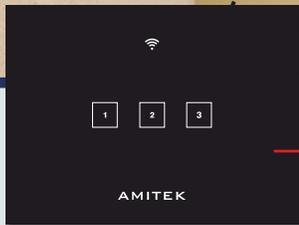
This capacitive touch glass panel is a user interface for controlling lights, fan, exhaust, etc.
